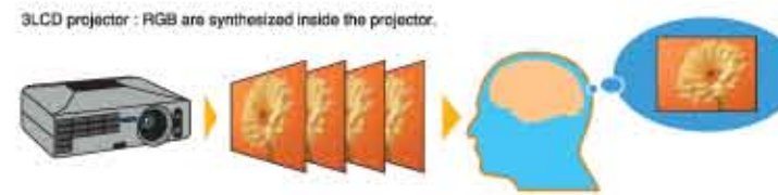
*HTPS(High Temperature Poly-Silicon) is an active matrix transmissive LCD. It is extremely small and produces high quality images.
